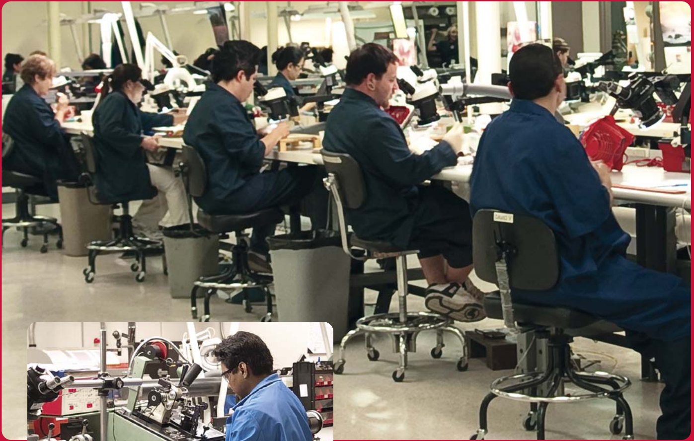
Left Precision winding equipment is used to insure compliance to customer specifications and tolerances. Above Microelectronics assembly lines dedicated to custom magnetics production.
