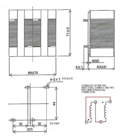
All dimensions are given In millimeters, unless otherwise specified, tolerance  $\pm 0.5$ mm
